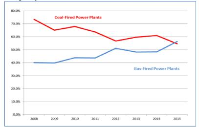
Figure 20: Capacity Factors of Gas-Fired Versus Coal-Fired Plants: 2008-2015
