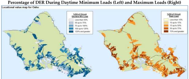
Figure 12: Density of Solar PV Systems on Electric Distribution Circuits Percentage of DER During Davtime Minimum Loads (Left) and Maximum Loads (Right)
